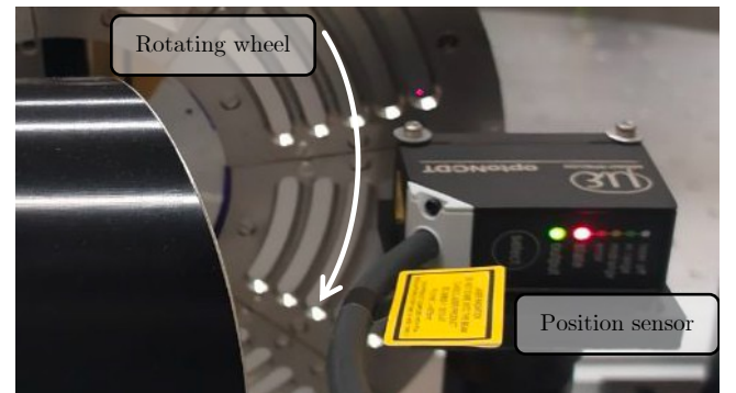
Figure 2. Picture of the setup used for the validation of the target positioning system.
