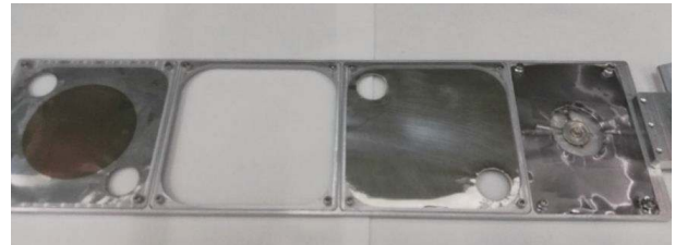
Fig. 2. Photo of the samples and the sample holder. In three of the four sample positions, the back-to-back ^{241}\text{Am} \alpha sources (right), the stainless steel sheet (second from right) and the ^6\text{LiF} samples (left) were installed.
