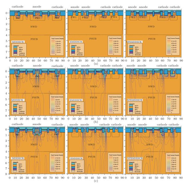
Fig. 4. Total current-flow-line at (a) the trigger point, (b) the holding point, and (c) the high ESD current pulse. In the legends of the figure,  $Si_3N_4$  and  $SiO_2$  symbolize  $Si_3N_4$  and  $SiO_2$  respectively. Number 3.43e + 04 equals to  $3.43 \times 10^4$ .
