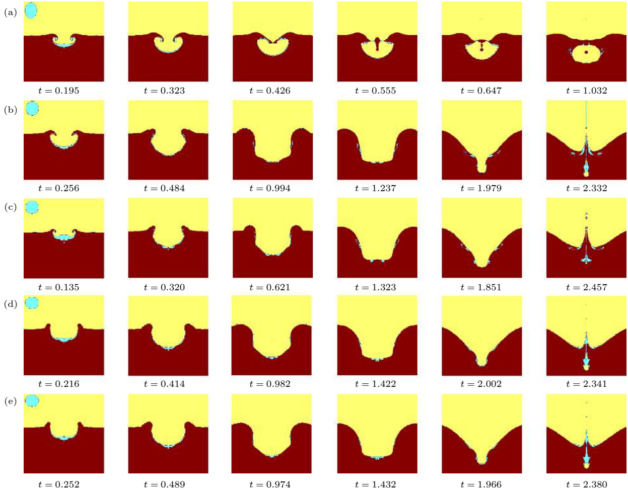
图 6 不同工况下自由液面随时间的运动过程 ( Fr = 112.5, We = 145, Re = 1740, V_i = 6 \text{ m/s} ) (a) AR = 1.33 ; (b) AR = 1.16 ; (c) AR = 1.00 ; (d) AR = 0.84 ; (e) AR = 0.67
