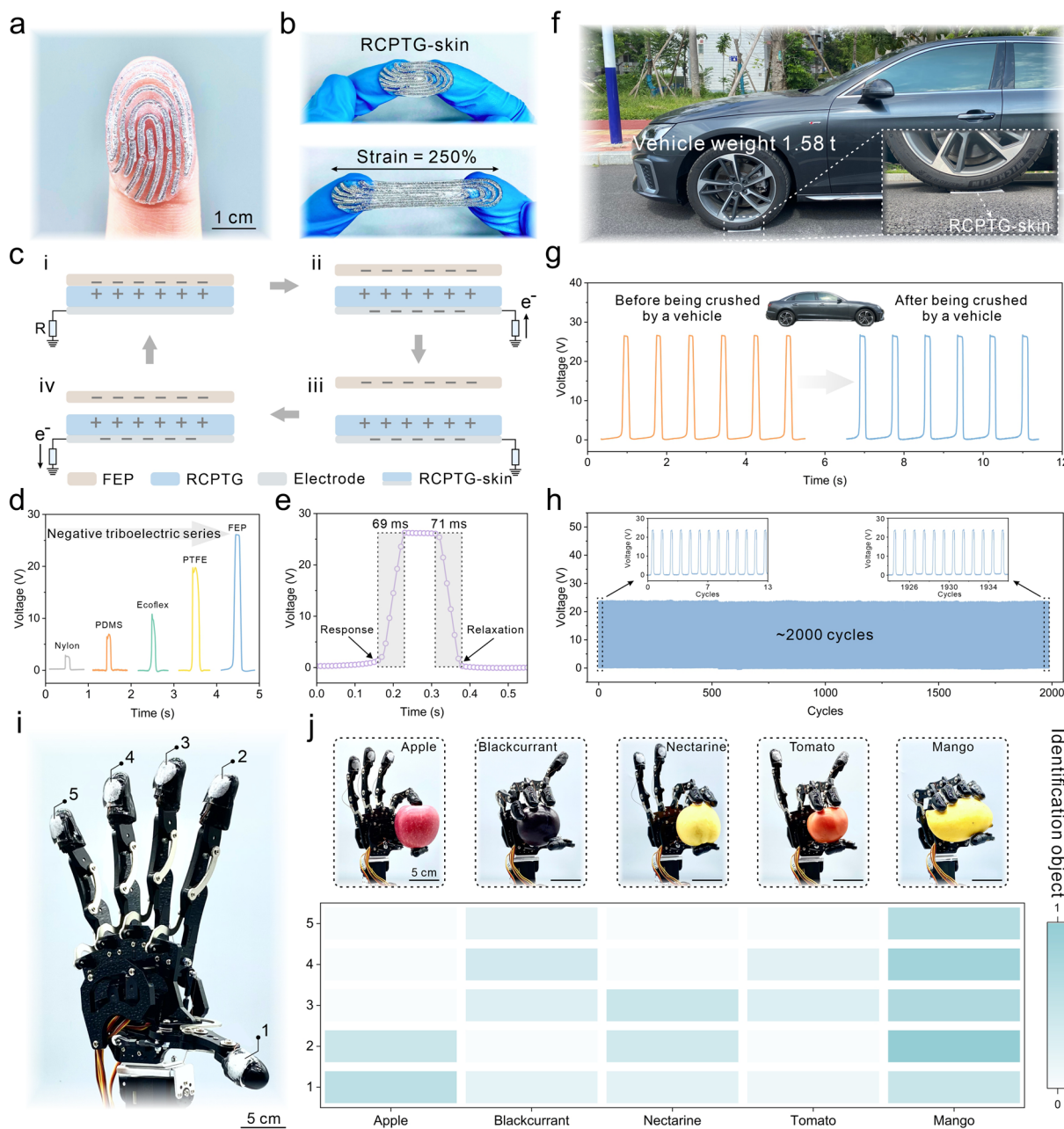
Fig. 5 Self-powered perception properties of triboelectric tactile skin. a Compliant RCPTG-skin configured on a finger. b Images of RCPTG-skin before (top) and after (bottom) being stretched. c Self-powered sensing mechanism of RCPTG-skin based single-electrode triboelectric nanogenerator. d Contact electrification properties of RCPTG-skin paired with different commercial materials. e Self-powered response and relaxation time of RCPTG-skin. f Image of RCPTG-skin when subjected to destructive crushing by a vehicle weighing 1.58 t. g Comparison of the triboelectric output of RCPTG-skin before and after crush. h Sensing stability of RCPTG-skin at ~2000 cycles. i Image of a triboelectric tactile sensory system. j A robotic hand integrated with self-powered tactile skin serves as an operable haptic gripper that recognizes grasping motions and strengths based on the magnitude of triboelectric signals
