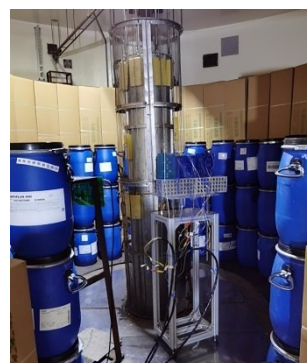
图1 器件总剂量辐照实验现场图 Fig.1 Picture of the device under 60 Co irradiation
