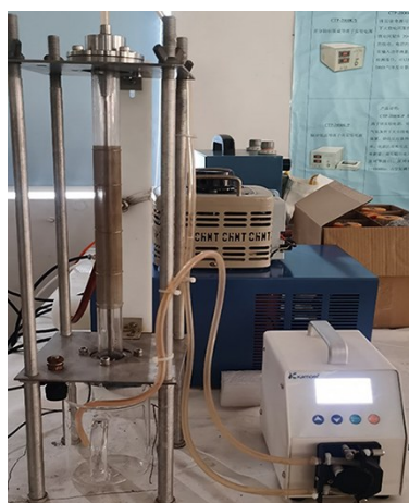
图1 同心管式介质阻挡放电低温等离子体反应器 Fig.1 Concentric tubular dielectric barrier discharge low-temperature plasma reactor
