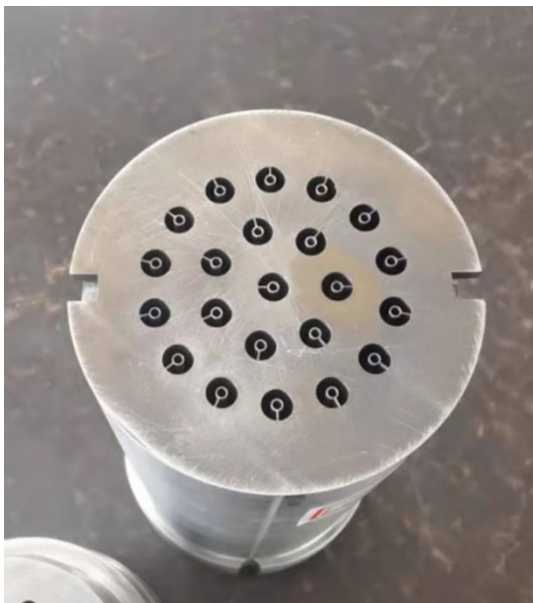
图6 锥形环孔式准直器实物图 Fig.6 Physical photo of conical pipe-embedded collimator
