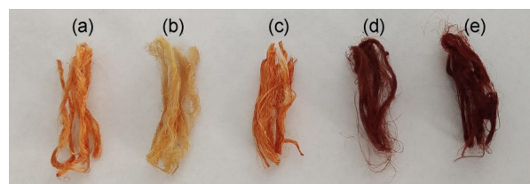
图2 (a) UHMWPE-PAA、(b) UHMWPE-PAM、(c) UHMWPE-PAA/NH 2 OH、(d) UHMWPE-PAM/NH 2 OH和(e) UHMWPE-HO吸附三价铁离子后的图片 Fig.2 Digital images of (a) UHMWPE-PAA, (b) UHMWPE-PAM, (c) UHMWPE-PAA/NH 2 OH, (d) UHMWPE-PAM/NH 2 OH, and (e) UHMWPE-HO after adsorption of Fe(III) ions
