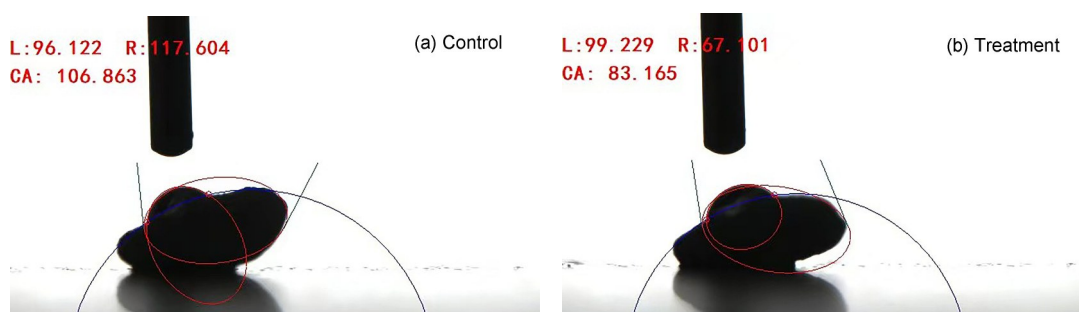
图6 接触辉光放电等离子体处理前后接触角测量图像:(a)对照组;(b)处理组;CA表示接触角 Fig.6 Contact angle measurement images before and after treatment with CGDP: (a) control; (b) treatment; CA stands for contact angle
