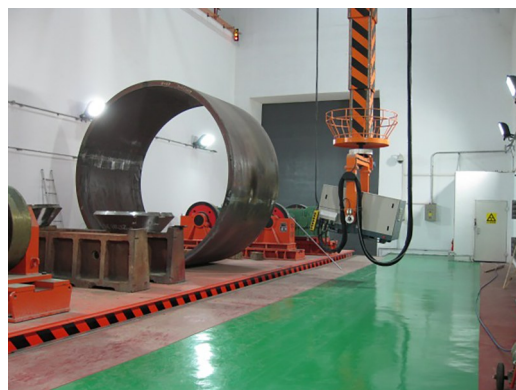
图2 无损检测用驻波电子直线加速器应用现场 Fig.2 Application scene of standing-wave electron linac for nondestructive testing
