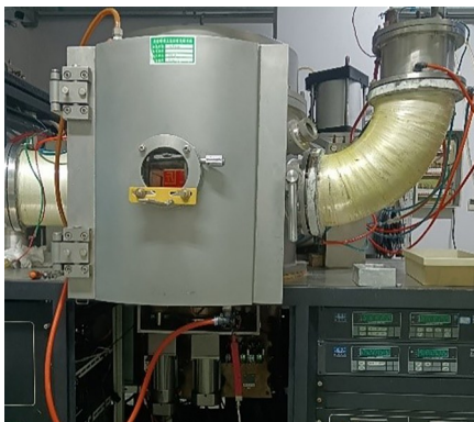
图7 磁过滤多弧离子镀膜设备(a)及磁过滤多弧离子镀膜设备原理图(b) Fig.7 Multi-arc ion plating equipment (a) and schematic diagram of magnetic filtration multi arc ion plating equipment (b)
