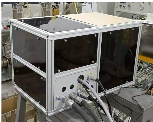
图3 6 MeV X波段驻波直线加速器的X射线头及微波单元 Fig.3 X-ray head and RF unit of 6 MeV X-band standing wave linac
