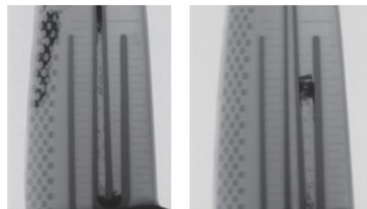
图 16 叶片残余型芯中子照相检测图像 [43] Fig.16 Inspection image of leaf residual core by neutron radiography [43]
