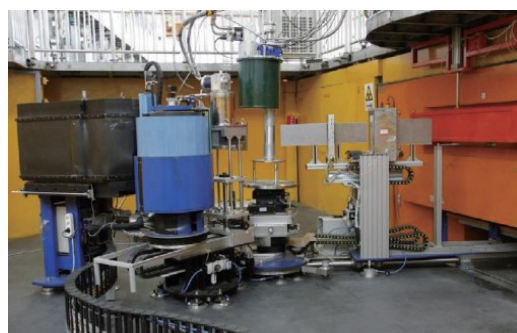
图10 冷中子三轴谱仪实物图 [38] (彩图见网络版) Fig.10 Snapshot of cold neutron triple-axis spectrometer [38] (color online)
