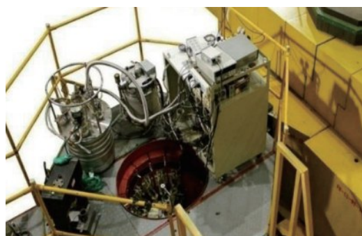
图11 高压中子衍射谱仪实物图 [39] (彩图见网络版) Fig.11 Snapshot of high pressure neutron diffractometer [39] (color online)
