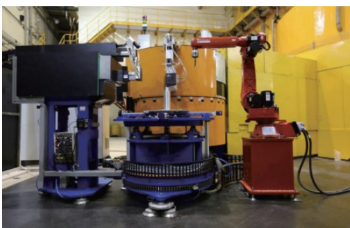
图8 中子应力谱仪实物图 [36] (彩图见网络版) Fig.8 Snapshot of residual stress neutron diffractometer [36] (color online)
