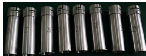
图 2 加工完成的典型辐照装置照片 Fig.2 Snapshot of typical irradiation device after processing
