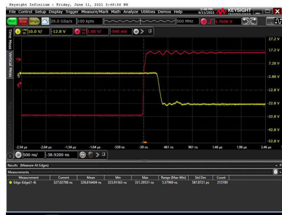
图9 单节点响应时间测试的示波器截图 Fig.9 Snapshot of oscilloscope results for single node response time test
