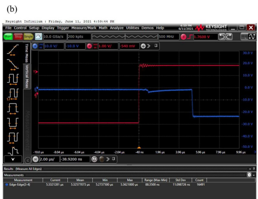
图10 节点间响应时间测试的示波器截图 (a) 1 m 电缆连接, (b) 800 m 电缆连接 Fig.10 Snapshot of oscilloscope results for multi-nodes response time test (a) 1 m cable connection, (b) 800 m cable connection
