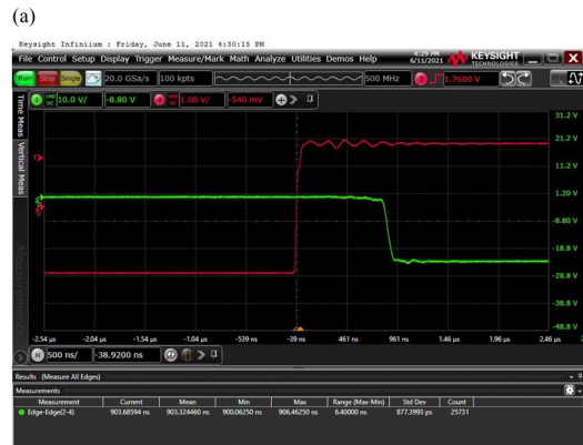
图9 单节点响应时间测试的示波器截图 Fig.9 Snapshot of oscilloscope results for single node response time test
