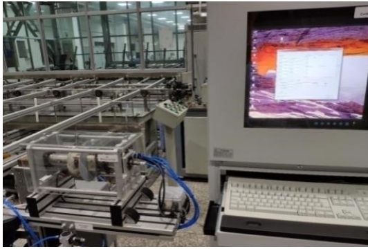
图3 燃料棒氦压无损检测设备实物图 Fig.3 Snapshot of non-destructive testing equipment for measurement of helium pressure inside fuel rod
