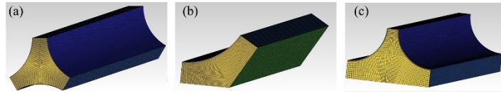
图2 内三角(a)、类五边形(b)和类梯形(c)通道网格划分 Fig.2 Mesh model of triangular channel (a), pentagonal channel (b) and trapezoidal channel (c)
