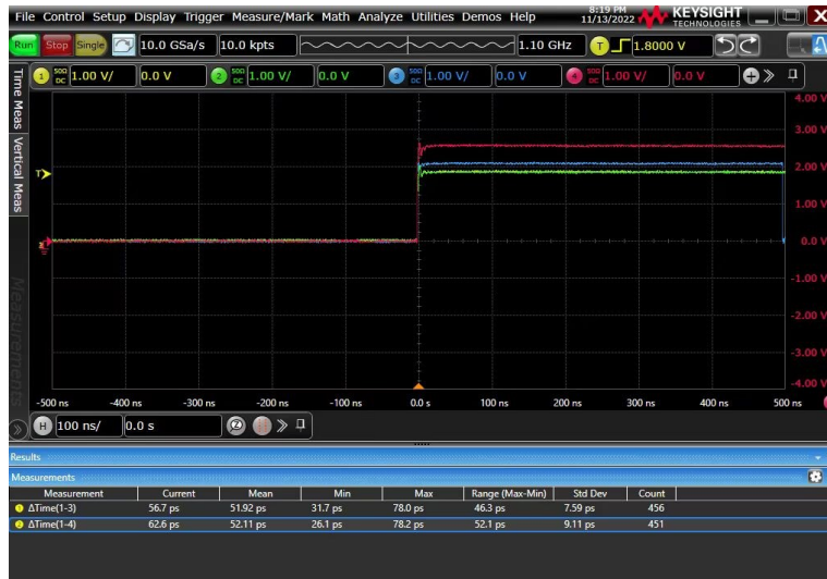
图6 SHINE 定时系统时间延迟测试结果截图 Fig.6 Snapshot of testing results of the time delay of the SHINE timing system
