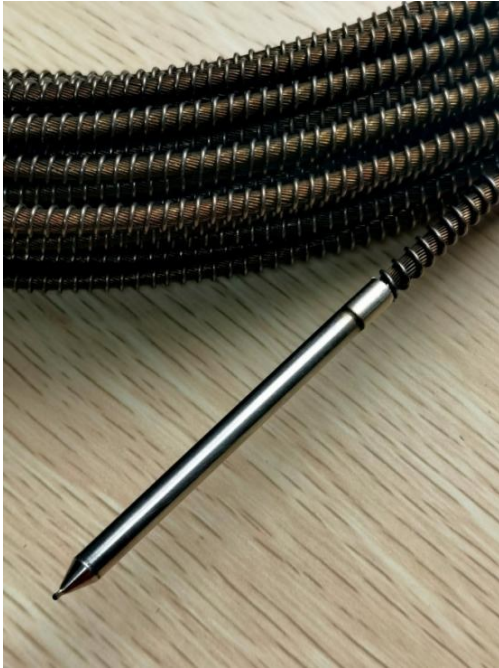
图2 移动式微型裂变室自研样机实物图 Fig.2 Snapshot of prototype for the mobile miniature-fission ionization chamber
