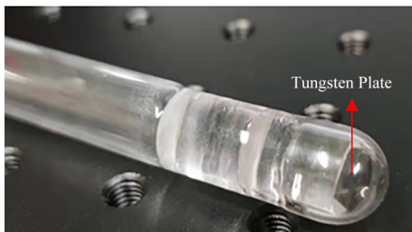
图 4 钨的真空密封 Fig.4 Snapshot of vacuum sealing of W
