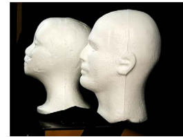
Fig. 2. Two life-size styrofoam heads used as test objects.
