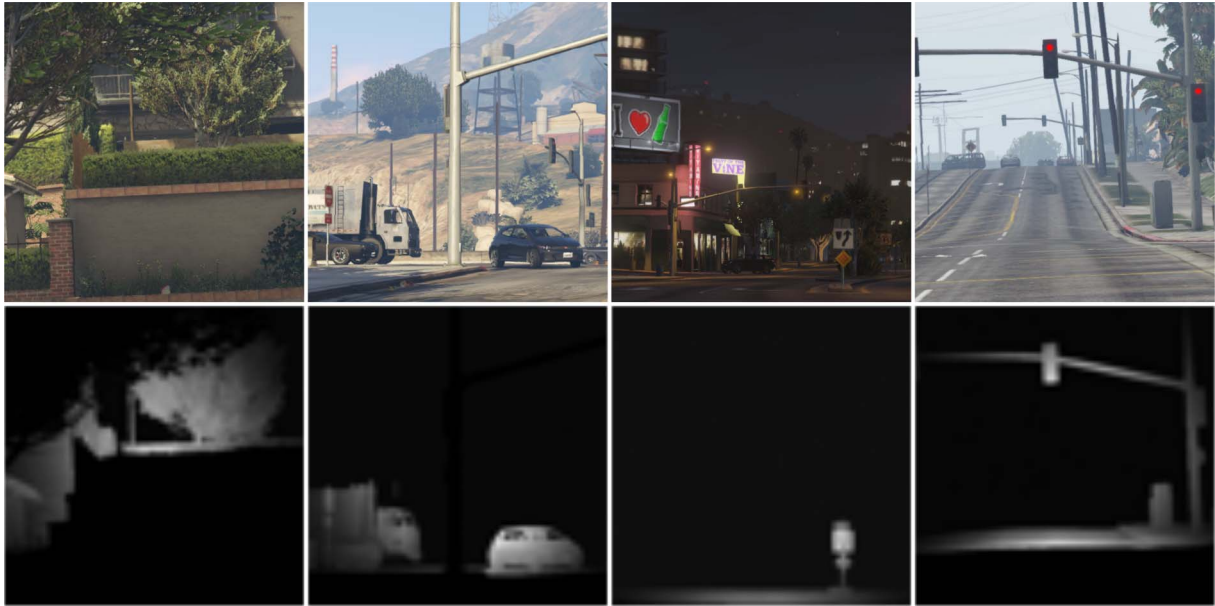
Fig. 2. Examples for image conversion: Original simulated RGB images (top row) and corresponding simulated foggy gated NIR images with active laser illumination (bottom). The original image size is 512 \times 512 pixels ( 13.3^\circ FOV) whereas the gated images are downsampled to 64 \times 64 pixels. The attenuation length of the fog was set to 13 m, the gate from 40 m to 60 m, the illumination FWHM to 6.4^\circ , the image blurring to one pixel (gaussian filter) and the background illumination to 1%. RGB images taken from [25].
