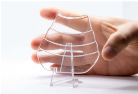
Fig. 5. Glass molded MODE lens ring segment using low transition temperature Ohara L-BSL7 glass.
