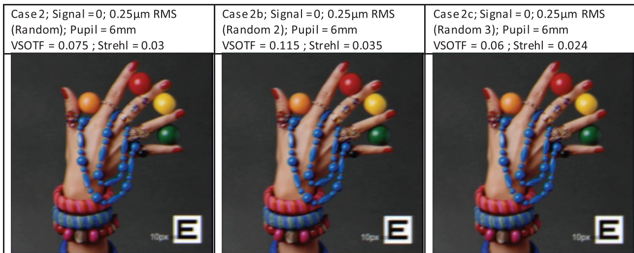
Fig. 14. Simulated retinal image and image quality metrics of three wavefronts comprising different set of randomly generated higher order (7–8th) Zernike coefficients as noise (RMS of 0.25 \mu m) fit to a 6 mm fit diameter.
