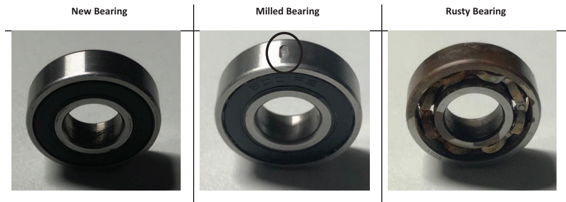
Figure 4. Left: new bearing, middle: bearing with milled structure and on the right handside a rusty bearing without grease.
