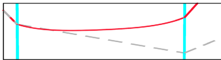
Fig. 8. Ray path within the middle lens without the consideration of \Delta n_\theta (grey, dashed) and with its consideration (red).
