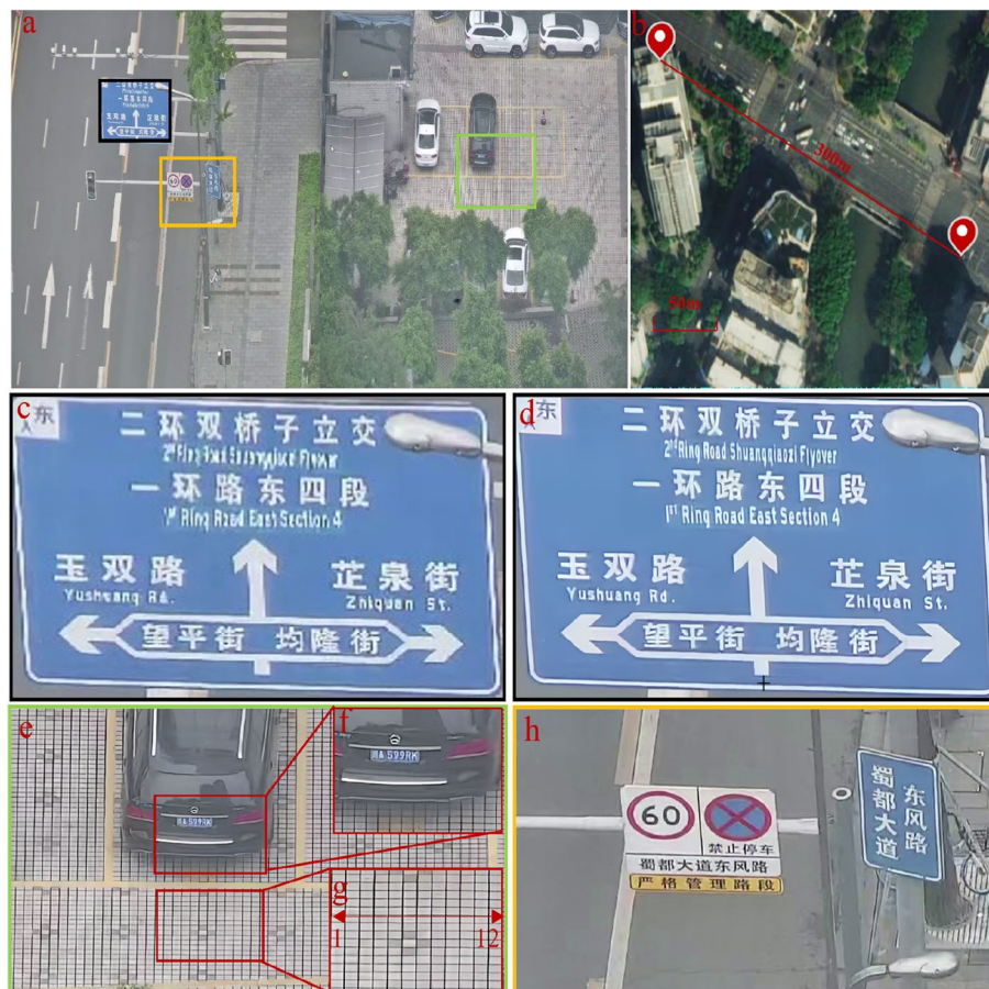
Fig. 5 SR interaction example with 4 \times computational zoom. a Wide-FOV example captured using 2 cameras of the DLBP camera. b Sky eye satellite map. Scale: 50 m. c Labeled region in Fig. 5a. d, e SR reconstruction examples with 4 \times computational zoom in Fig. 5a. f, g enlarged images in Fig. 5e. h SR reconstruction examples with 4 \times computational zoom in Fig. 5a
