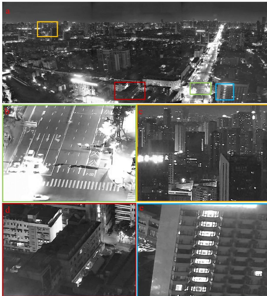
Fig. 9 Interactive panorama example in the infrared band, covering 0.3–4 km. a Infrared panorama captured using the DLBP camera, which is stitched by 6 sub-images. b–e Infrared-SR reconstruction images with 4x computational zoom, which is one-to-one corresponding to the label area in Fig. 9a
