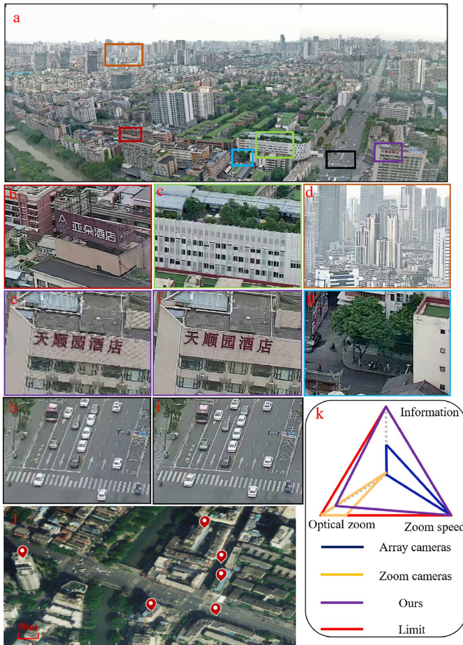
Fig. 4 Interactive panorama example captured using the DLBP camera. a Stitched panorama, which is stitched by 6 sub images. b-d SR reconstruction images with 4 × computational zoom. e Labelled region from panorama f-g SR reconstruction images with 4 × computational zoom, which recovers the rich information from short-focus to long-focus imaging. h Labelled region from panorama. i SR reconstruction image with 4 × computational zoom. j Sky eye satellite map. k Comparison of ours with the conventional systems.
