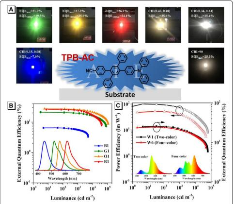
**Fig. 2 a** Molecular structure of TPB-AC and EL performances for nondoped OLED, PhOLEDs and WOLEDs based on TPB-AC. **b** and **c** EQE – luminance curves of nondoped OLED, PhOLEDs and WOLEDs; inset: EL curves for the OLEDs. Reprinted with permission from ref. [34] Copyright 2019 American Chemical Society
