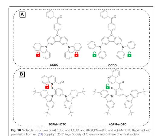
The doped OLED fabricated by 2QPM-mDTC could afford high maximum EQE, CE and PE of 24.0%, 79.5 cd  $A^{-1}$  and 62.3 lm  $W^{-1}$ , respectively.
