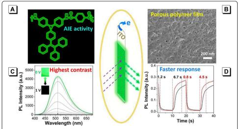
**Fig. 20 a** The molecular structure of PA-TPE; **b** SEM (scan electron microscope) image of PA-TPE-0.03 film; **c** PL spectra changes of PA-TPE thin film at different potentials (inset shows the optical images of polymer film under excitation of 365 nm with applied potential of 0 and 1 V, respectively); **d** Fluorescence switching response under applied potentials of PA-TPE. Reprinted with permission from ref. [102] Copyright 2018 American Chemical Society
