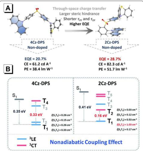
**Fig. 11 a** The molecular configurations of 2Cz-DPS and 4Cz-DPS. **b** Energy level diagrams, spin–orbital coupling constants (ξ) and non-adiabatic coupling effects of 2Cz-DPS and 4Cz-DPS. Reprinted with permission from ref. [67] Copyright 2019 Royal Society of Chemistry
