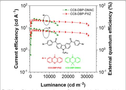
**Fig. 12** Current efficiency–luminance–external quantum efficiency characteristics of the nondoped devices. Configurations: ITO/PEDOT:PSS (50 nm)/PVK (30 nm)/emitter/TmPyPB (40 nm)/LiF (1 nm)/Al. Reprinted with permission from ref. [70] Copyright 2019 Royal Society of Chemistry
