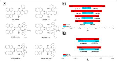
**Fig. 13 a** The molecule structures of *R/S*-BN-CF, *R/S*-BN-CCB, *R/S*-BN-DCB, *R/S*-BN-AF, (*R*)-OBN-Cz and (*S*)-OBN-Cz. **b**. The  $g_{\text{EL}}$  values of doped and neat films. Reprinted with permission from ref. [75] Copyright 2018 Wiley-VCH
