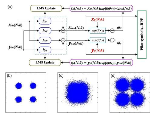
**Fig. 3** Equalization algorithm process and constellations of the encrypted and decrypted QPSK signal. (a) Jointly LMS equalization and phase noise compensation by pilot symbols; (b) constellation of decrypted QPSK signals in the back-to-back case; (c) constellation of chaotic encrypted carrier; (d) constellation of decrypted QPSK signal by NN after 800 km fiber transmission.
