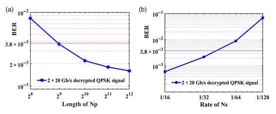
**Fig. 5** BER performance. BER performance of decrypted QPSK signal after 800-km fiber transmission (a) with the length of  $N_p$  and (b) with the pilot rate of  $N_s$ .
