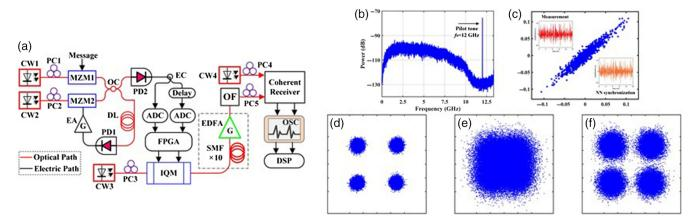
**Fig. 4** Experimental setup and results of real-time pilot-based coherent chaotic fiber transmission system. (a) Experimental setup; (b) pilot tone structure of chaotic encrypted carriers; (c) plot of chaotic time series collected from PD2 and NN synchronization; (d) constellation of decrypted QPSK signals in the back-to-back case; (e) constellation of chaotic encrypted carrier; and (f) constellation of decrypted QPSK signal by NN after 800 km fiber transmission.
