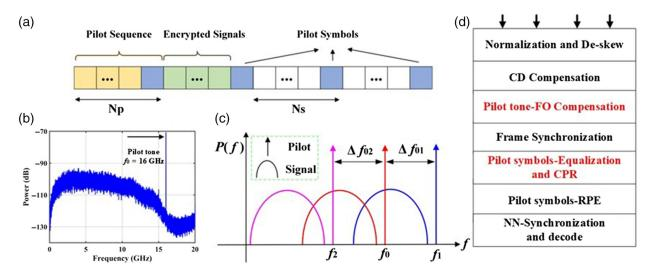
**Fig. 2** Pilot structure at the transmitter and the DSP module at the receiver. (a) Frame structure of pilot symbols; (b) pilot tone structure of chaotic encrypted carriers; (c) principle of FO compensation by pilot tone; and (d) receiver pilot-based DSP module. CD, chromatic dispersion; CPR, carrier phase recovery; RPE, residual phase estimation; and NN, neural network.
