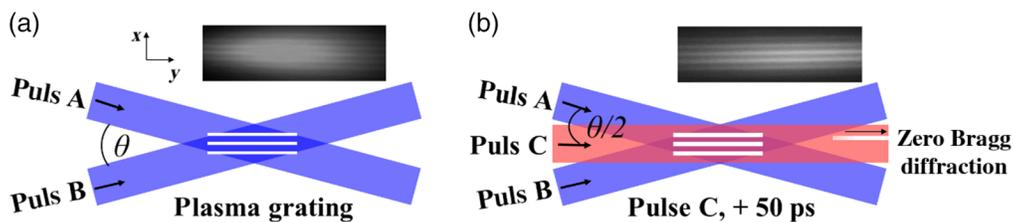
**Fig. 4** Top view of the noncollinear interaction area between pulses A and B to create plasma gratings (a) without and (b) with the third filament (pulse C) entering the plasma grating at 50 ps delay, respectively. The plasma grating fluorescence photos are shown in the inset pictures.
