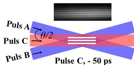
**Fig. 5** Top view of the noncollinear interaction area between the ahead pulse C ( $-50$  ps delay) and plasma grating inducing by pulses A and B.
