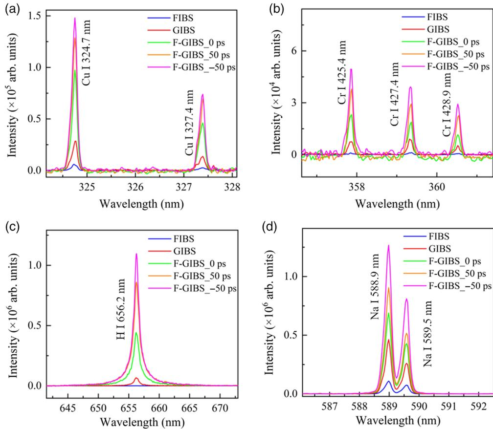
**Fig. 7** Comparison of FIBS, GIBS, and F-GIBS at different delays (0 and  $\pm 50$  ps) in aqueous solutions for spectral lines of (a) Cu, (b) Cr, (c) H, and (d) Na elements.
