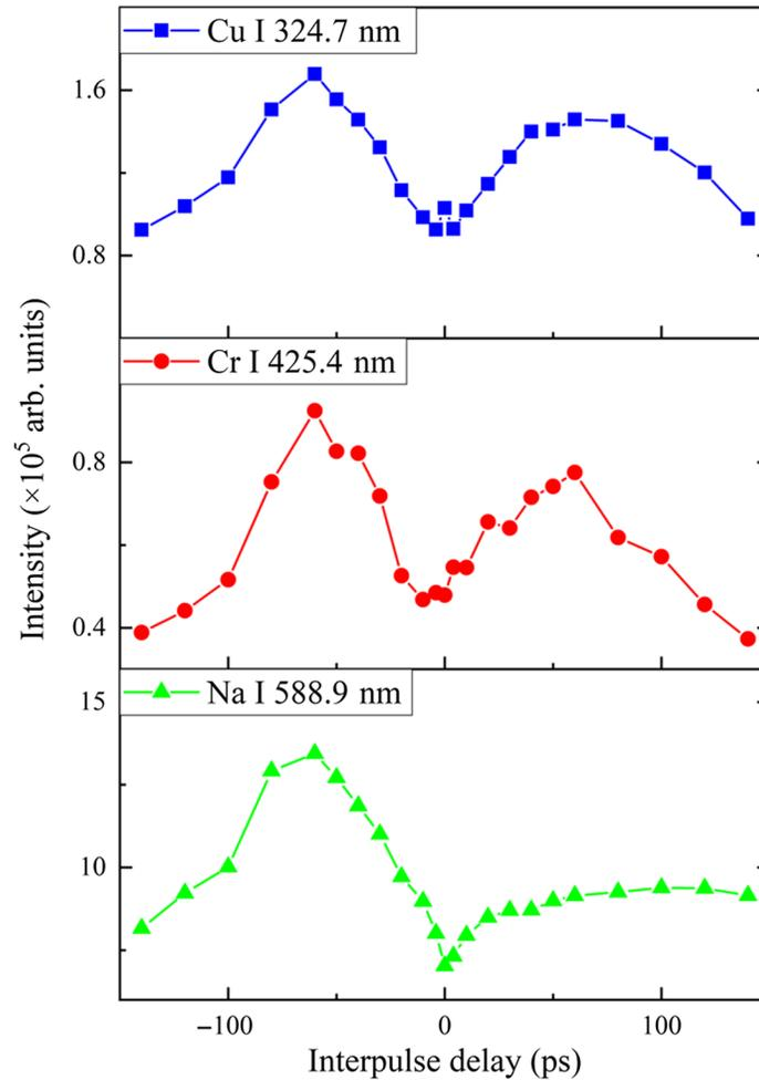
**Fig. 3** F-GIBS signals of Cu I 324.7, Cr I 425.4, and Na I 588.9 nm attained under different interpulse delays.
