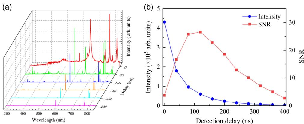
**Fig. 2** Time evolution of a typical F-GIBS spectrum: evolution of (a) a typical F-GIBS with the detection delay and (b) the intensity and SNR of Cu I 324.7 nm excited by F-GIBS.
