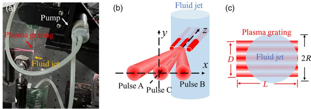
**Fig. 1** (a) Photo of plasma-grating excited fluid jet stream. (b) Schematic of the spatial configuration of three filaments generated by pulses A, B, and C. The parallel structure represents plasma gratings generated by the nonlinear interactions of coplanar filaments A, B, and/or C. (c) Schematic of the top view of the plasma grating interacting with the fluid jet.
