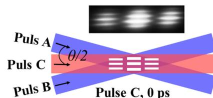
**Fig. 6** Top view of the noncollinear coplanar filament interaction area as the three filaments are synchronized.
