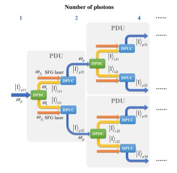
**Fig. 1** Scheme for deterministic *N*-photon state generation using the PDU. As marked in a gray box, a PDU is used to convert a pump photon to a biphoton with the same frequency deterministically, through nondegenerate DPDC and DPUC processes. By cascading the PDUs, the photon number can be doubled exponentially, toward deterministic generation of an *N*-photon state, with the Fock state as an example.
