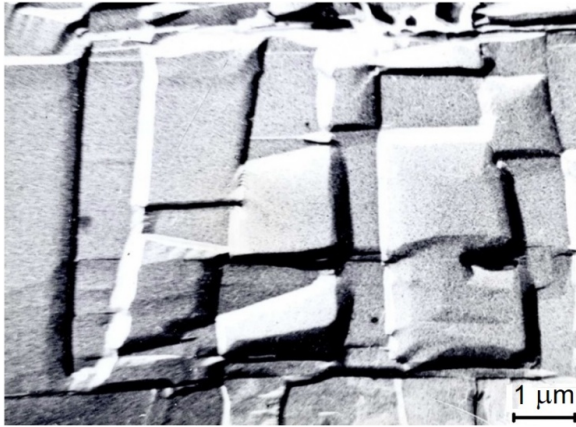
Fig. 3. Real domain structure in TB-2 ceramics: 90° structure with a substructure along the a-component, wall along (001).
