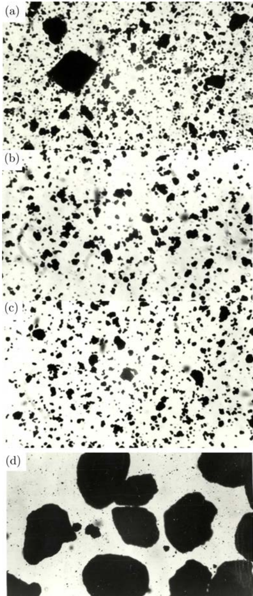
Fig. 1. (a) Powder obtained by grinding a porous framework, \times 330 , (b) powder obtained by grinding a porous framework with following chemical treatment and annealing, \times 330 , (c) powder obtained by processing the synthesized material with a KCl melt, \times 330 , (d) powder obtained by firing granular synthesized material, \times 45 .
