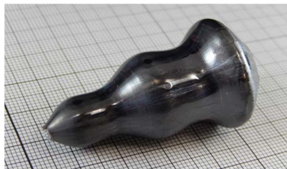
Fig. 2. Photograph of as-grown BCT single crystal.
