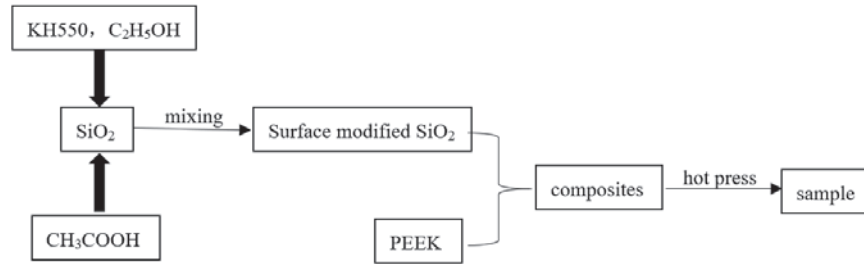
Fig. 2. Flow chart for the preparation of SiO 2 -PEEK composites.
