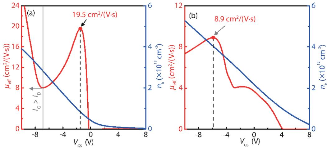
Fig. 4. (Color online) The  $\mu_{\text{eff}}$  and the  $n_h$  of (a) Si-rich and (b) N-rich sample with  $\sim 48$  nm trench.
