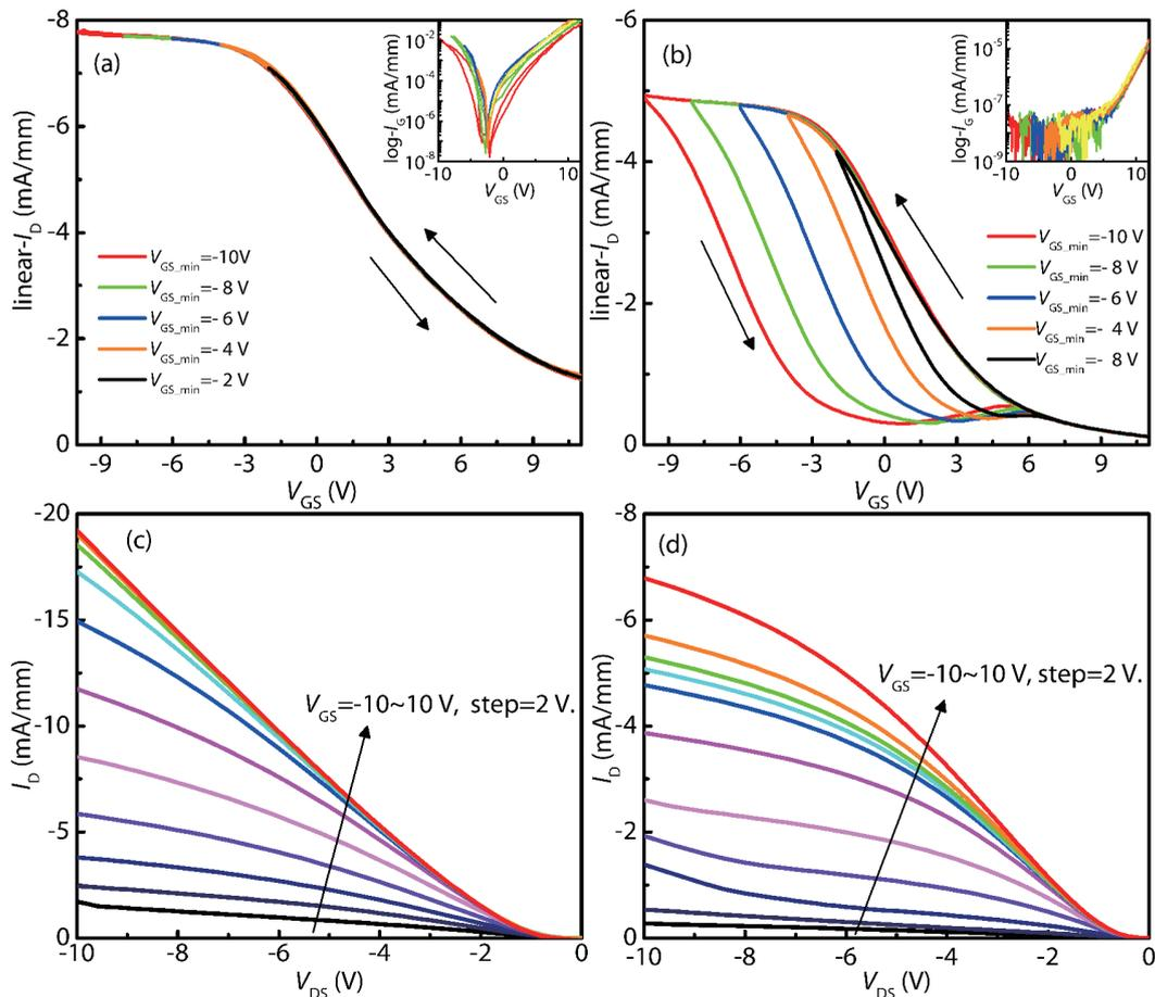
Fig. 3. (Color online) The transfer characteristic of (a) Si-rich sample and (b) N-rich sample. The output characteristic of (c) Si-rich sample and (d) N-rich.
