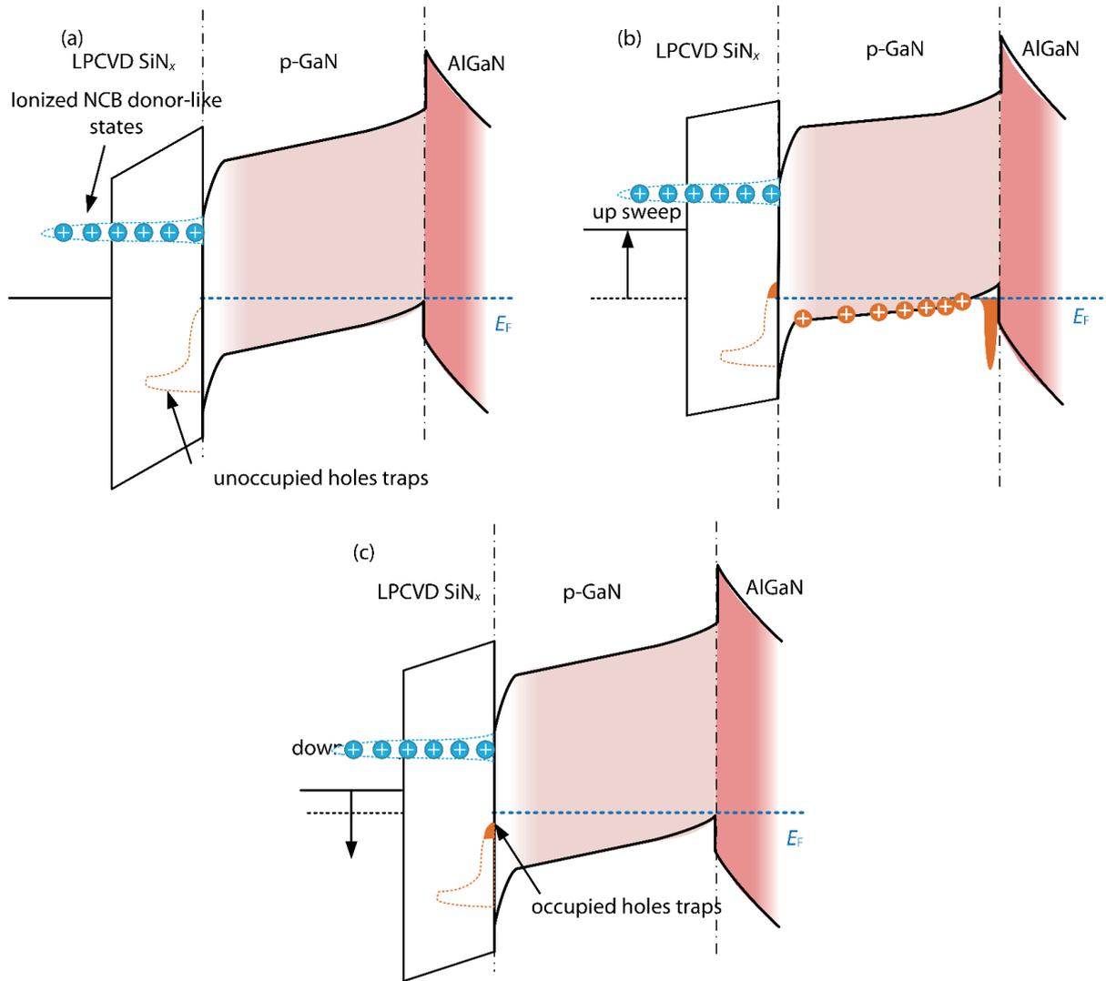
Fig. 8. (Color online) The Band diagram schematics of the MIS gate of Si-rich sample during the (a) initial state, (b) up sweep and (c) down back.
