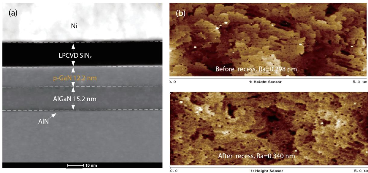
Fig. 5. (Color online) (a) The focused ion beam section of  $\sim 12$  nm channel. (b) The surface morphology characterized before/after recess.
