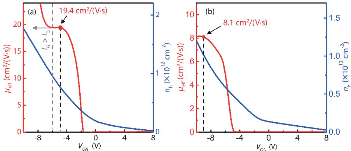
Fig. 10. (Color online) The  $\mu_{\text{eff}}$  and the  $n_h$  of (a) Si-rich and (b) N-rich sample with  $\sim 58$  nm trench.
