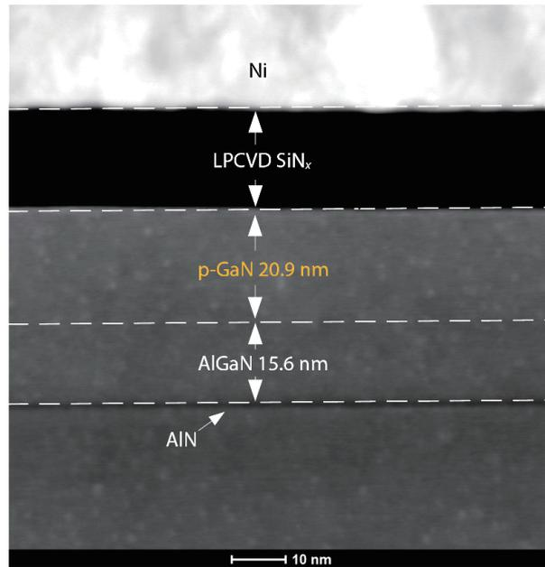
Fig. 2. (Color online) The focused ion beam section of  $\sim 22$  nm channel.
