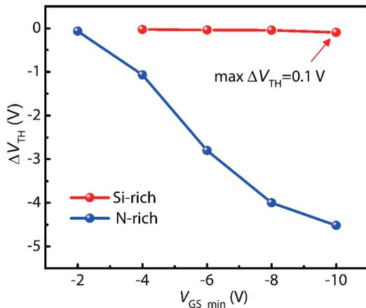
Fig. 7. (Color online) The  $\Delta V_{TH}$  with different  $V_{GS}$  sweep ranges.
