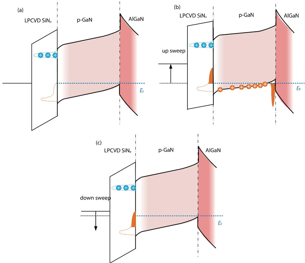
Fig. 9. (Color online) the Band diagram schematics of the MIS gate of N-rich sample during the (a) initial state, (b) up sweep and (c) down back.
