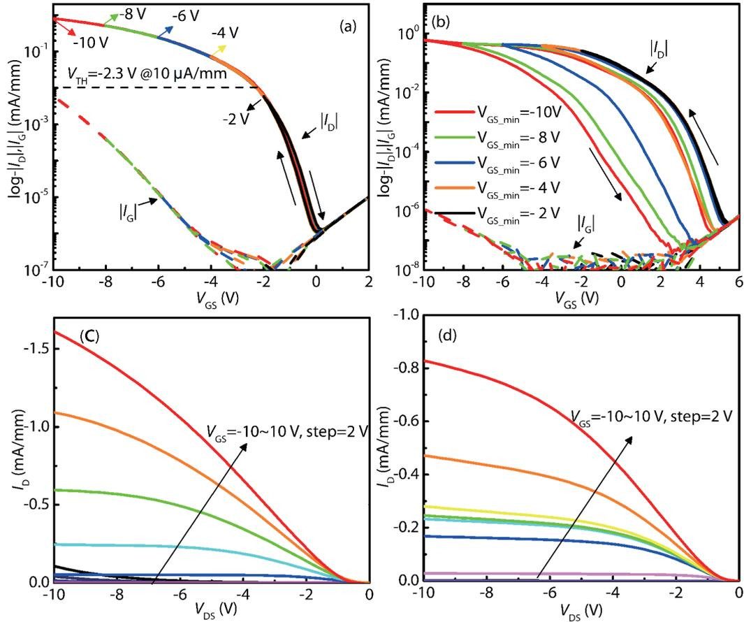
Fig. 6. (Color online) The transfer characteristic of (a) Si-rich sample and (b) N-rich sample. The output characteristic of (c) Si-rich sample and (d) N-rich.
