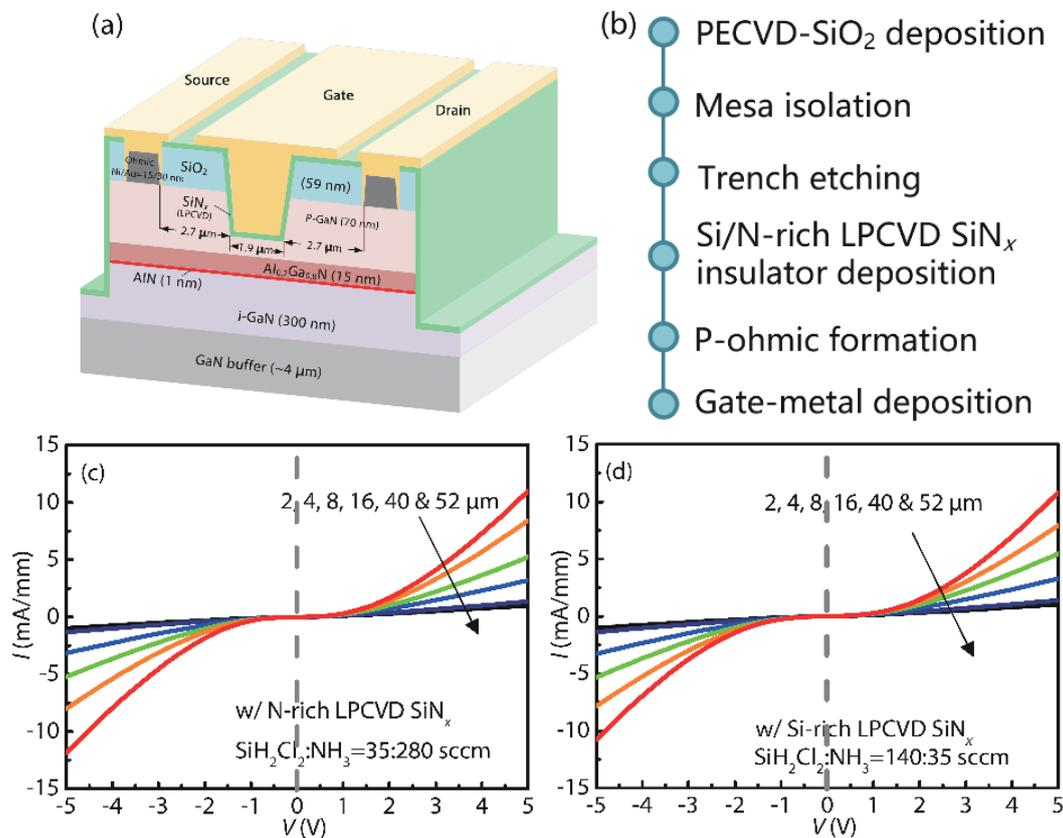
Fig. 1. (Color online) (a) Epitaxial structure and schematic of the proposed device. (b) The fabrication procedure. The  $I$ - $V$  characteristic measured from TLM for the samples with (c) N-rich LPCVD  $\text{SiN}_x$  and (d) Si-rich LPCVD  $\text{SiN}_x$ .
