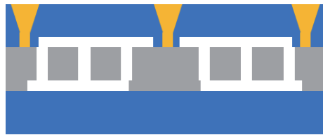
Fig. 4. (Color online) Package with anodic bonding.
