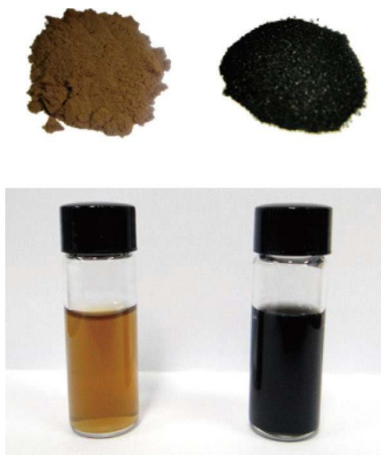
Fig. 14. (Color online) Image of powder and the aqueous dispersion of graphene oxide (0.5 mg/mL) before (left) and after reduction (right) [104] .
