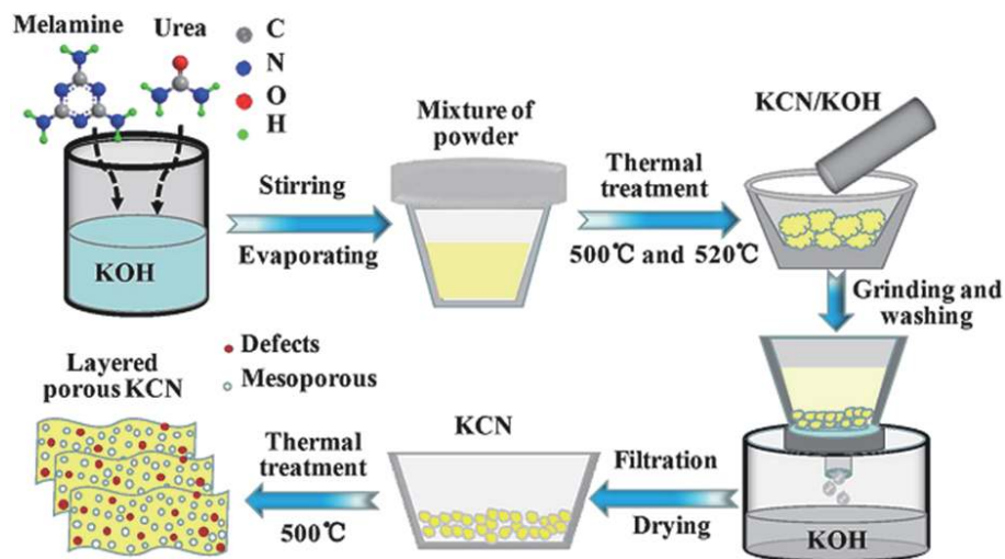
Fig. 4. (Color online) Schematic illustration of synthesis methods of DTLP-CN via thermal polymerization of melamine, urea, and KOH. Reprinted from Ref. [25].
