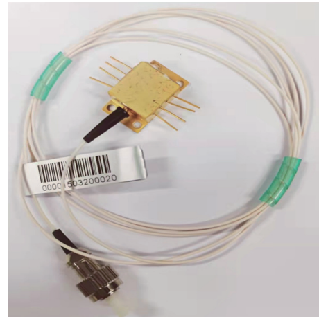
Fig. 7. (Color online) Dual SPADs balanced detector with fiber-coupled package.
