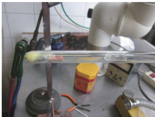
Fig. 1. The ampoule containing the constituent elements of CZTS under evacuation.
