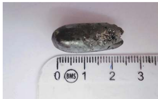
Fig. 2. The obtained ingot of CZTS.
