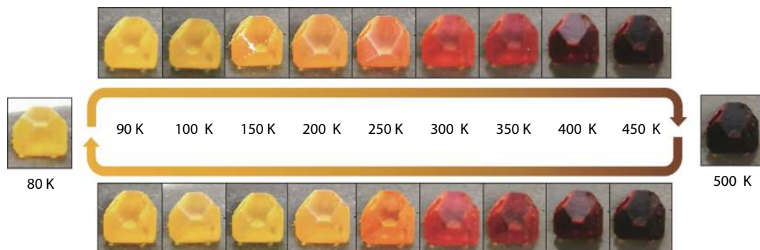
Fig. 1. (Color online) Colour evolution of as-prepared \text{Cs}_2\text{NaFeCl}_6 single crystal as the function of temperature in the range of 80–500 K.
