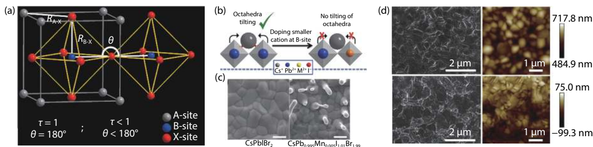
Fig. 6. (Color online) (a) Relation of the tolerance factor ( \tau ) with a B–X–B bond angle ( \theta ) of the ABX_3 perovskite structure. Reproduced with permission [88] . Copyright 2018, American Chemical Society Publications. (b) Rotational distortion of [BX_6]^{4-} ( [PbX_6]^{4-} ) octahedra can be restricted by reducing the B–X bond length when Pb^{2+} is partially substituted with smaller B-site cations. Smaller B-site cations reduce the size of the [BX_6]^{4-} octahedron, which in turn decreases the size of the cuboctahedral void for the A-site cation. Reproduced with permission [88] . Copyright 2018, American Chemical Society Publications. (c) Typical SEM images of CsPbBr_2 , and CsPb_{0.995}Mn_{0.005}Br_{1.99}I_{0.01} films, respectively. Reproduced with permission [91] . Copyright 2018, Wiley-VCH Publications. (d) SEM images of (above) CsPbBr_2I and (below) CsPb(Ba)Br_2I . Reproduced with permission [93] . Copyright 2017, Elsevier Inc Publications.
