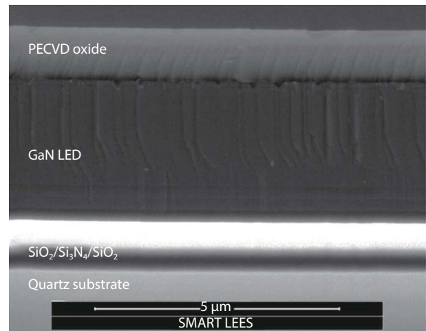
Fig. 34. SEM image of the cross-sectional view of the bonded GaN LED on the quartz substrate.
