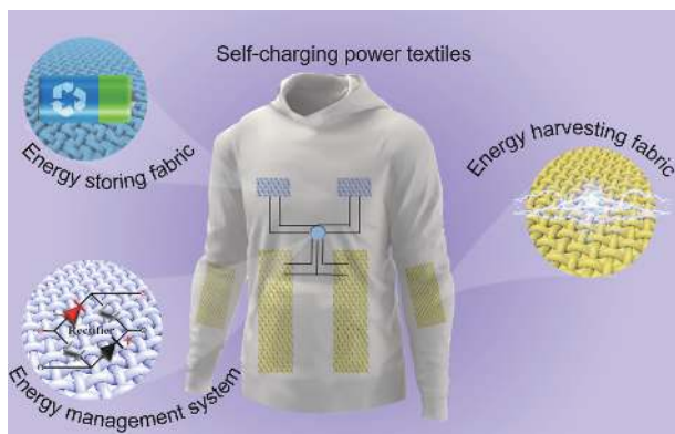
Fig. 1. (Color online) Schematic illustration of self-charging power textiles, mainly including fiber/fabric-based energy harvesting units, fiber/fabric-based energy storage unit, and power management circuits.
