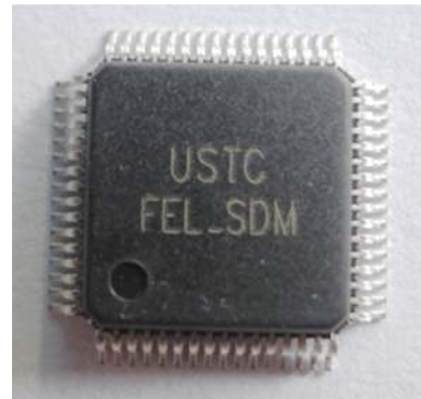
Fig. 16. \Sigma - \Delta modulator (SDM) layout architecture and chip after manufacturing.
