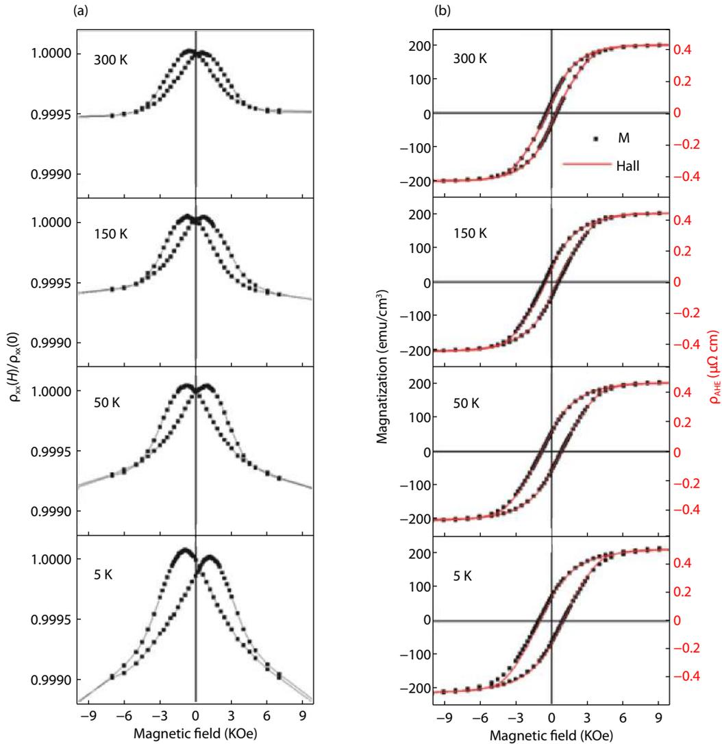
Fig. 8. (Color online) (a) Normalized MR and (b) anomalous Hall resistivity and corresponding M-H loops for the  $\text{Ga}(\text{Co}_{0.4}\text{Zn}_{0.6})_{0.98}\text{O}$  film from room temperature down to 5 K. Reprinted with permission from Ref. [102]. Copyright (2017) by AIP Publishing.
