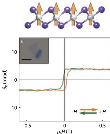
Fig. 5. (Color online) (a) Out-of-plane view of the  $\text{CrI}_3$  structure depicting the Ising spin orientation. (b) Polar MOKE signal for a  $\text{CrI}_3$  monolayer at a temperature of 15 K. The inset shows an optical image of an isolated monolayer (the scale bar is  $2 \mu\text{m}$ ). Reprinted with permission from Ref. [87]. Copyright (2017) by Springer Nature.
