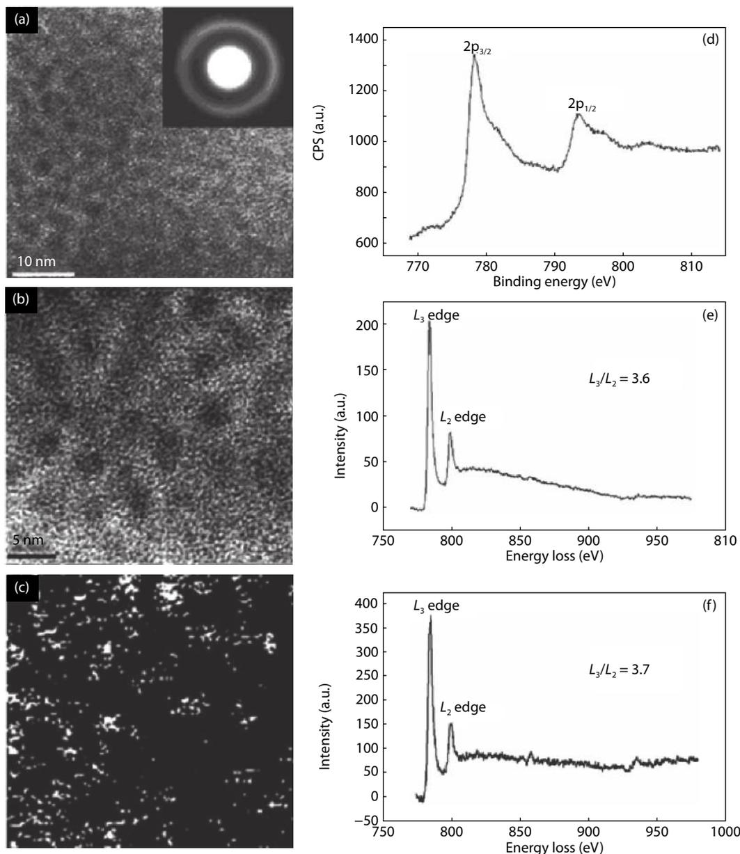
Fig. 10. (a) A low magnification micrograph of  $\text{Ti}_{0.24}\text{Co}_{0.76}\text{O}_2$  films and the corresponding electron diffraction pattern in the inset. (b) The high resolution TEM image, and (c) the corresponding elemental mapping of Co. (d) XPS of Co  $2p_{3/2}$  and Co  $2p_{1/2}$  peaks. (e) Electron energy-loss spectroscopy of  $\text{Ti}_{0.24}\text{Co}_{0.76}\text{O}_2$  films. Reprinted with permission from Ref. [106]. Copyright (2006) by AIP Publishing.
