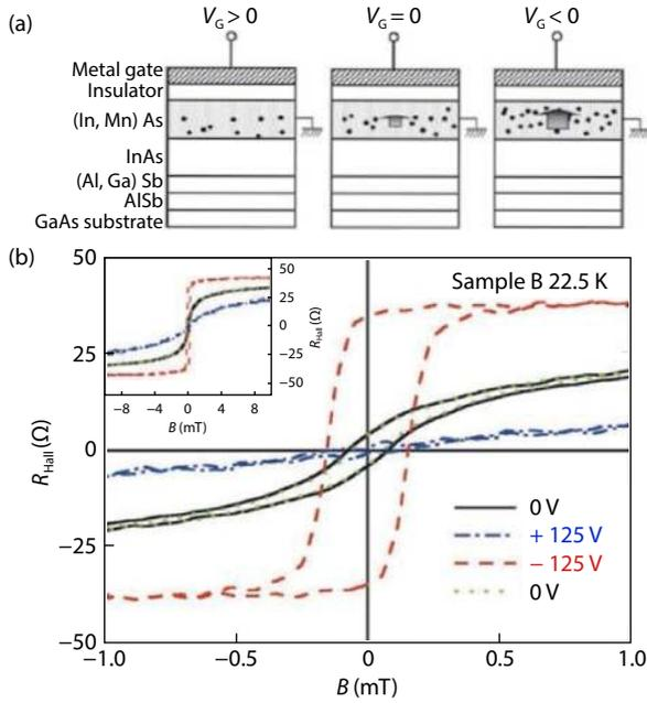
Fig. 2. (Color online) (a) Electric field control of the hole-induced ferromagnetism in magnetic semiconductor (In,Mn)As field-effect transistors. (b) Hall resistance versus field curves under three different gate biases. Inset, the same curves shown at higher magnetic fields. Reprinted with permission from Ref. [19]. Copyright (2000) by Springer Nature.
