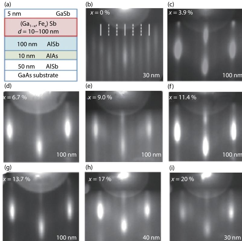
Fig. 6. (Color online) (a) Schematic fabrication of  $(\text{Ga}_{1-x}\text{Fe}_x)\text{Sb}$  thin films. (c)–(i) RHEED patterns taken along the  $[\bar{1}10]$  azimuth after the MBE growth of the  $(\text{Ga}_{1-x}\text{Fe}_x)\text{Sb}$  layers for samples A–G ( $x = 3.9\%$ – $20\%$ , thickness  $d = 30$ – $100$  nm). The RHEED pattern of an undoped GaSb sample is also shown as a reference in (b). Reprinted with permission from Ref. [99]. Copyright (2015) by AIP Publishing.
