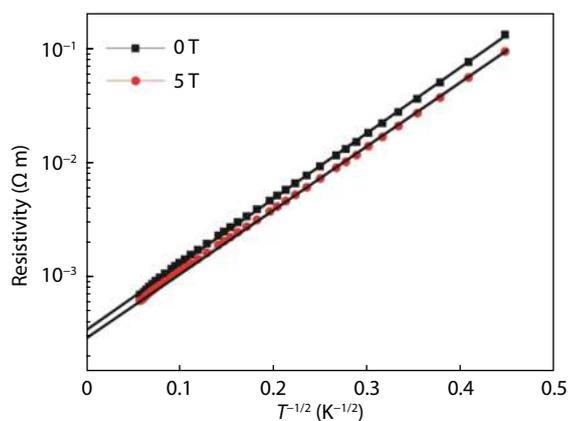
Fig. 11. (Color online) Resistivity in logarithmic scale versus  $T^{-1/2}$  for the  $\text{Zn}_{0.31}\text{Co}_{0.69}\text{O}_{1-v}$  magnetic semiconductors measured at zero and 5 T magnetic field. Reprinted with permission from Ref. [108]. Copyright (2010) by AIP Publishing.
