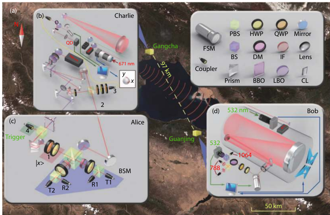
Fig. 13. (Color online) (a) Bird's-eye view of experiment site in China. (b–d) Illustration of the entangled photon pair generation and distribution from Charlie, single photon state preparation and Bell state measurement from Alice and single photon state reconstruction from Bob. Reprinted with permission from Ref. [119]. (Springer Nature)
