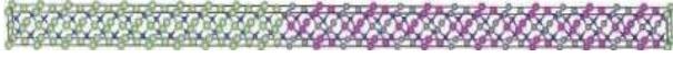
Fig. 1. (Color online) The crystal structure of superlattice GaX/ZnGeX 2 (X = N, P, As, Sb). The Ga, Zn, Ge and X atoms are in light green, purple, gray and blue, respectively.
