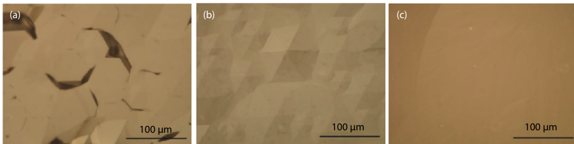
Fig. 10. (Color online) Nomarski micrographs of AlN layers: (a) directly growth, (b) two-step (c) three-step [54] .
