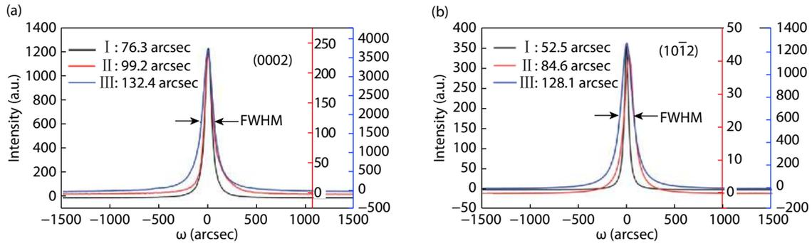
Fig. 3. (Color online) HRXRD of AlN samples (a) (0002) plane and (b)  $(10\bar{1}2)$  plane.
