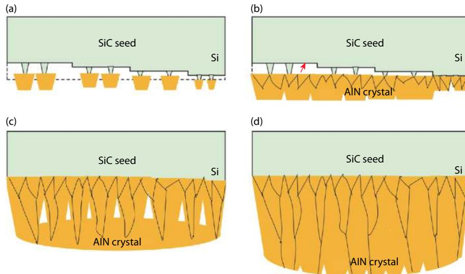
Fig. 4. (Color online) Schematic diagrams of AlN single crystal grown on Si-polar SiC seed. (a) SiC macroscopic steps and deposited AlN 3D islands. (b) AlN 3D islands lateral overgrowth and dislocation formation. (c, d) Cavity movement and dislocation "annihilation".
