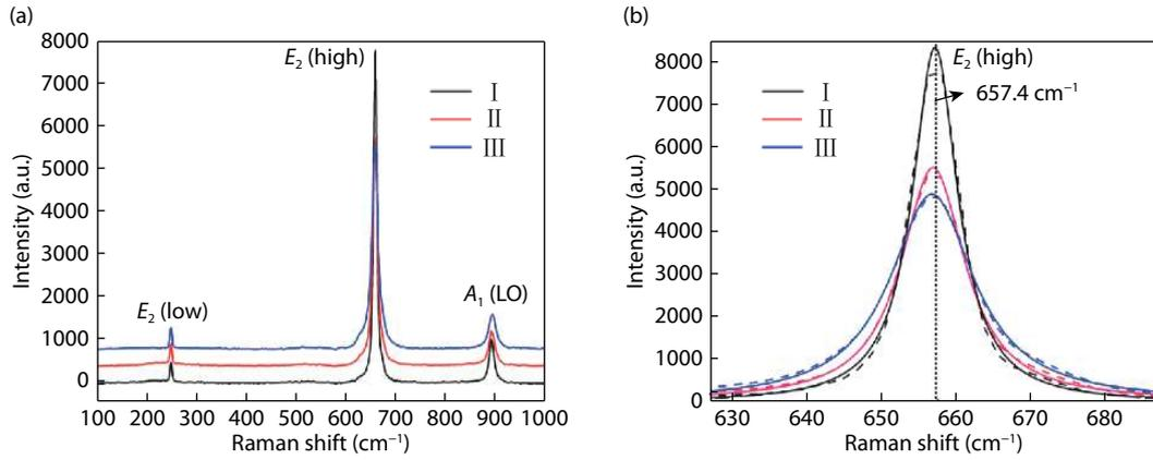
Fig. 2. (Color online) Raman spectrum of AlN samples. (a) Wavelength from 100 to 1000 nm. (b) Detailed  $E_2$  (high) phone mode peaks.
