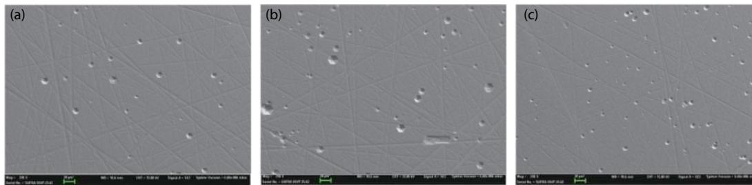
Fig. 5. SEM images of AlN samples etched in KOH/NaOH melt solution at 320 °C for 3 min. (a) Sample I. (b) Sample II. (c) Sample III.
