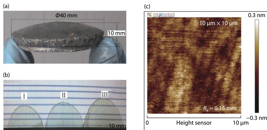
Fig. 1. (Color online) (a) AlN single crystal. (b) AlN samples. (c)  $R_a$  of AlN sample at area of  $10 \times 10 \mu\text{m}^2$ .
