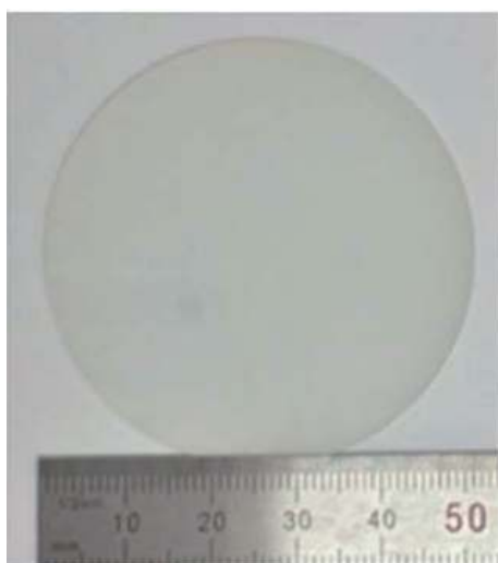
Fig. 14. (Color online) Photograph of a freestanding GaN substrate by in situ removal Si substrate.
