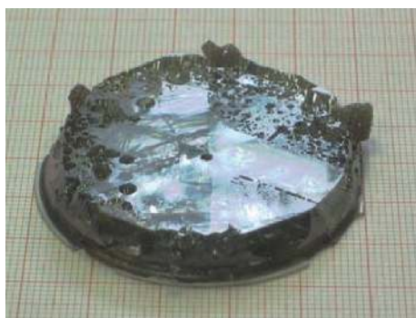
Fig. 4. (Color online) Photograph of a 6.3 mm thick GaN boule grown by Aixtron vertical HVPE.
